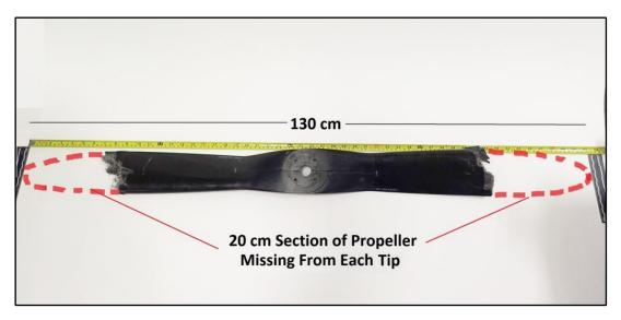
Photo No. 2: Damaged carbon fibre propeller
